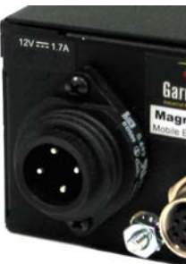
Fig 3.4b Dual-Source DC power input
