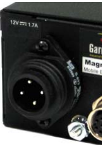
Fig 3.4a Single DC power input
