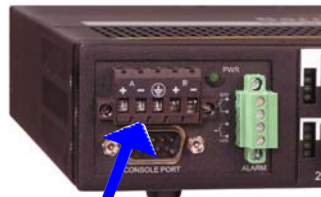
Terminal Block for DC Power
