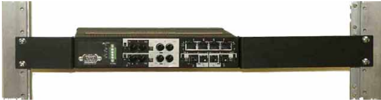
One 6K16 may be rackmounted, as shown above, using Model# K16-RMB brackets.
