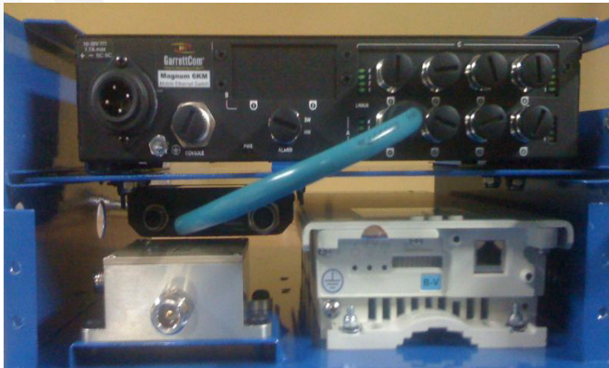
Magnum 6KM Mobile Ethernet Switch, wireless radio in NEMA 4 enclosure
